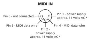
\*: AC voltage is routed to Pin 1 and Pin 2 only when the Phantom Power switch is engaged.
